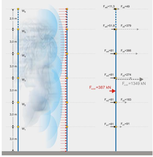
Figure 2.5-2: Wind forces  $F_w$  are less significant comparing to earthquake forces  $F_s$ . W [kN]: gravity loads  $F_w [kN]$ : wind forces  $F_s [kN]$ : seismic forces
