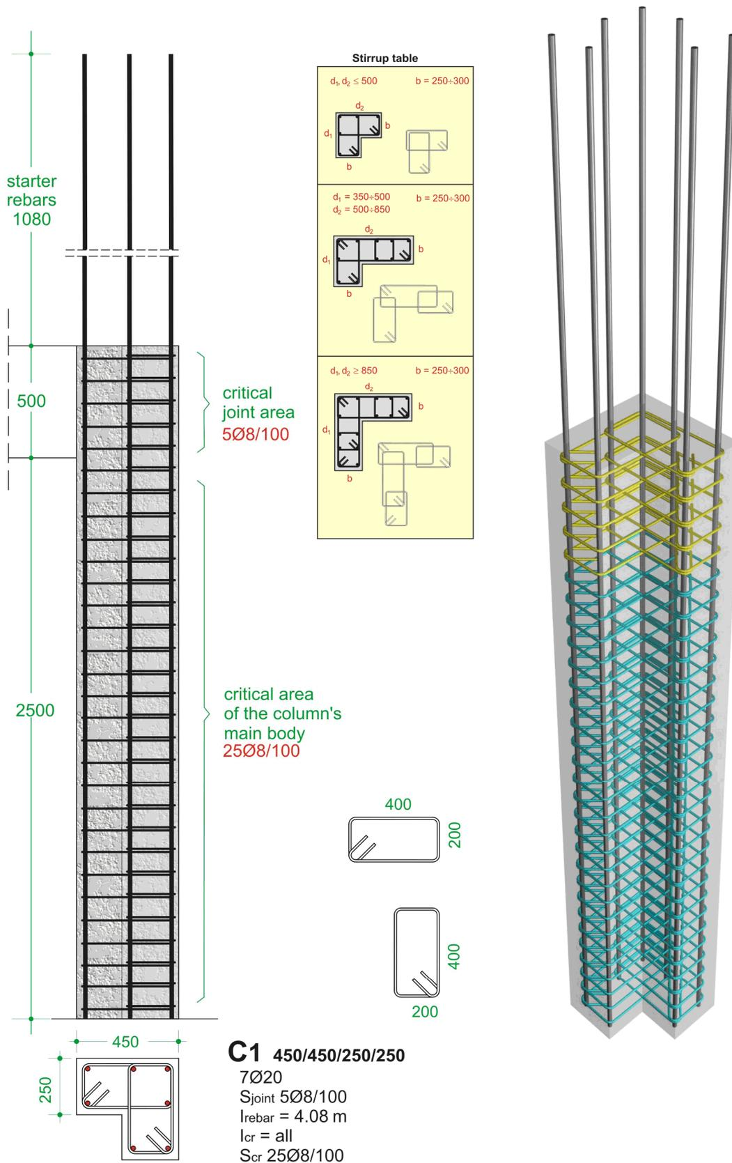
**Column with 'Γ' section 400x800x250x250 mm**
