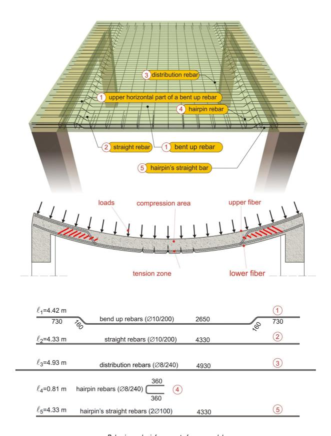
Behavior and reinforcement of one-way slab
