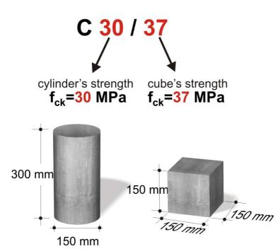
classification of concrete The grades is based on their compressive strength. Each concrete grade (Concrete) e.g. C30/37 is characterized two equivalent by strengths, which in this specific example are 30 MPa and 37 MPa. The first is the characteristic strength f<sub>ck</sub> of a standard concrete cylinder4 and the latter is the characteristic strength of a standard concrete cube.
