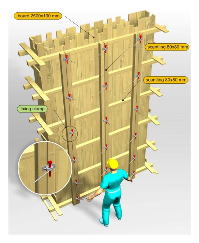
The mould elements might be conventional or industrialized. The former are mainly made out of natural timber and based on their section dimensions they are called:
