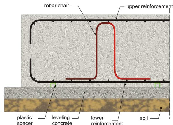
The reinforcement of a solid raft foundation can be separated into three categories, as shown at the following figure:
