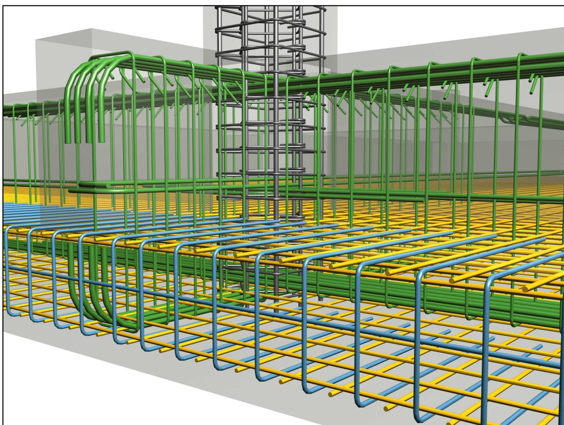
*Reinforcement of a ribbed raft foundation*
