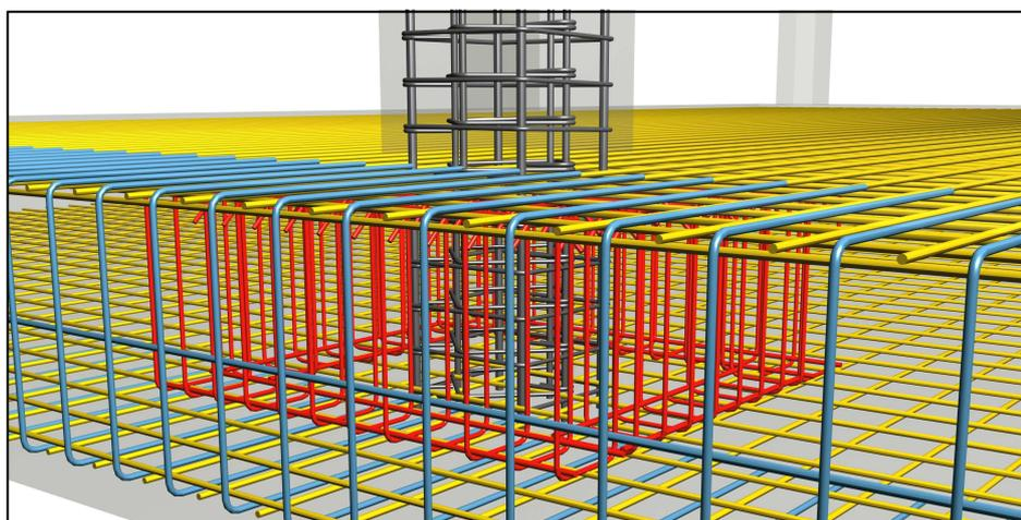
*Raft foundation with punching shear reinforcement*
