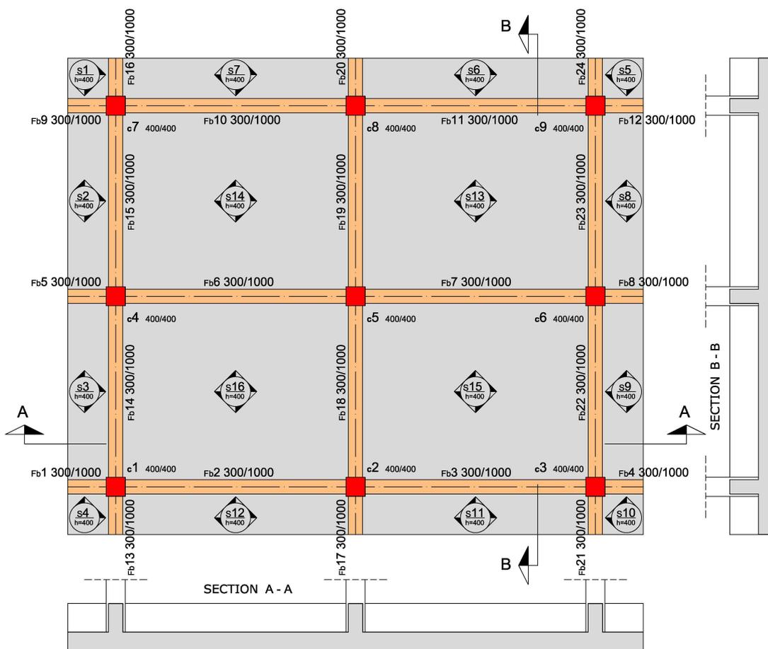
Unified foundation slab (raft foundation) with stiffeners (beams)
