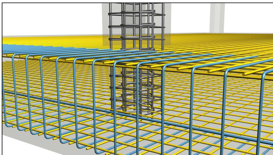
*Reinforcement of a solid raft foundation*
