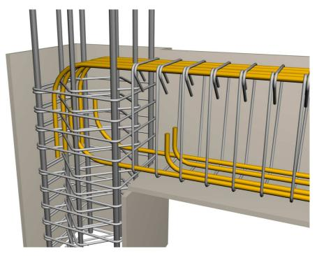
Anchorage with drum in a small sized column.
