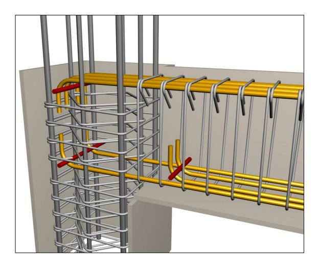
As far as the bar anchorage for slabs or beams is refereed to as 'simple hook anchorage' then metal pins should be placed in the bending areas with a diameter  $\geq \emptyset$
