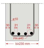
Self Compacting Concrete Beam **4Ø20** Stirrups Ø10 Coating =30 mm
