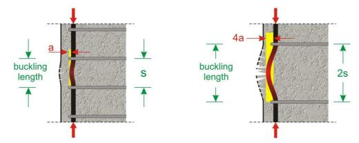
In a seismic event, columns always fail in the same way:
