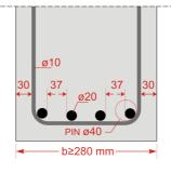
Usual Concrete Beam 4Ø20 Stirrups Ø10 Coating =30 mm
