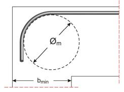
In columns that have a small dimension in the anchorage direction, (see the table below) the bending is implemented with the use of a large diameter drum.
