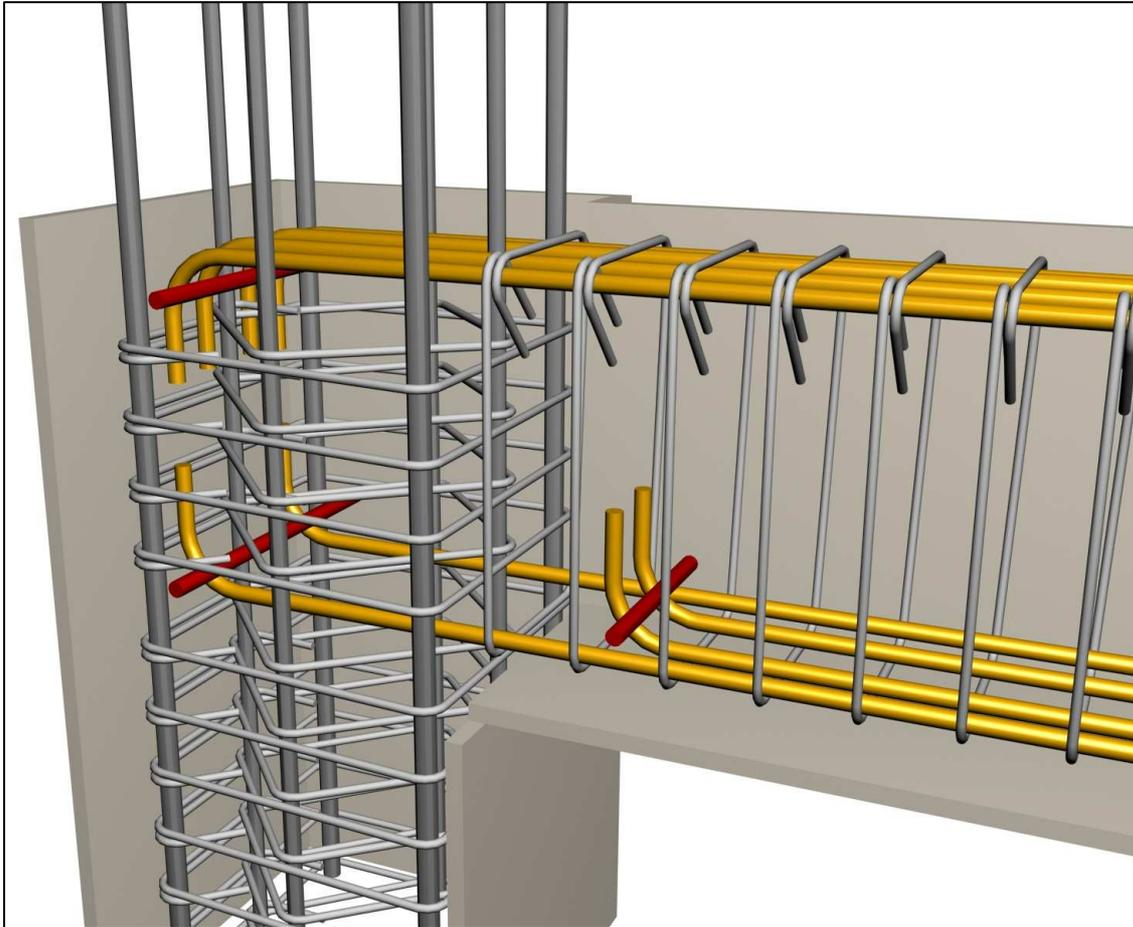
*As far as the bar anchorage for slabs or beams is referred to as 'simple hook anchorage' then metal pins should be placed in the bending areas with a diameter  $\geq \emptyset$*
