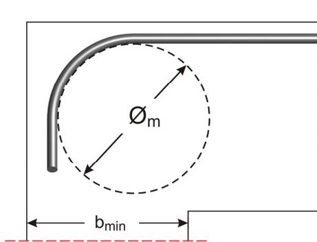
In columns that have a small dimension in the anchorage direction, (see the table below) the bending is implemented with the use of a large diameter drum.
