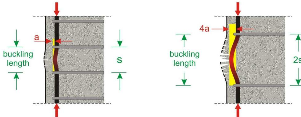
In a seismic event, columns always fail in the same way:
